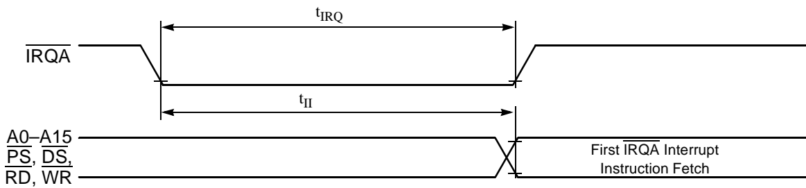
Figure 18. Recovery from Stop State Using \overline{\text{IRQA}} Interrupt Service
