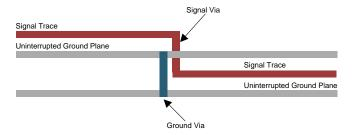
Figure 24. Ground Via Location (Side View)
