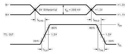
Figure 10. Receiver Propagation Delay and Transition Time Waveforms
