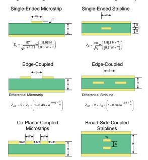
Figure 14. Controlled-Impedance Transmission Lines
