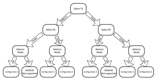
Figure 11. Deskew Configuration Setup Chart
