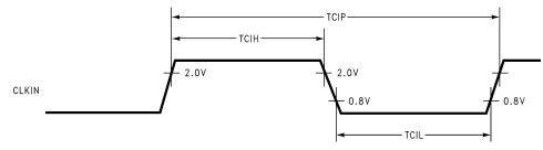
Figure 4. Input Clock High/Low Times
