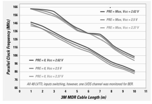
Figure 13. Data Rate vs Cable Length
