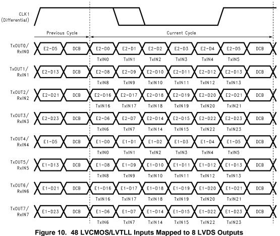
(DC Balance Mode- Enabled; BAL = High) (E1 - Falling Edge; E2 - Rising Edge)
