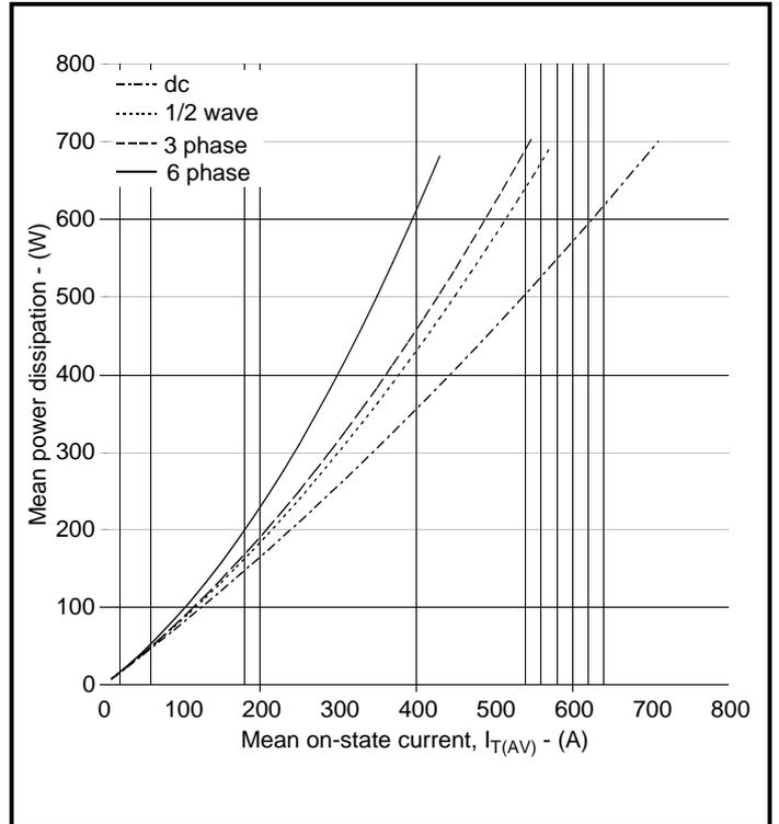
**Fig.3 Dissipation curves**
