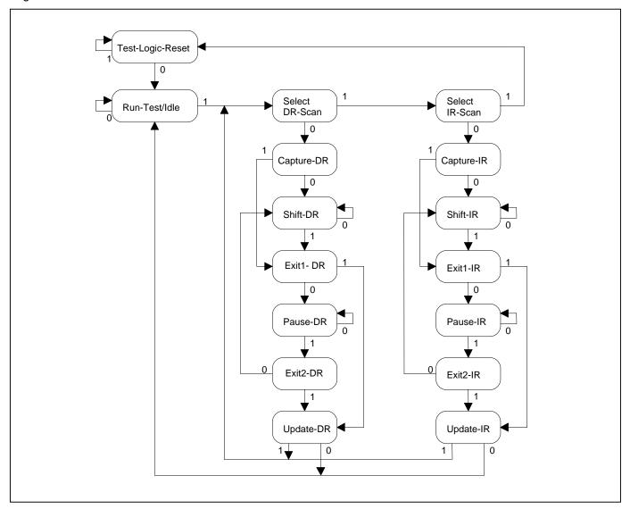
**Test-Logic-Reset.** Upon device power-up, the TAP controller starts in the Test-Logic-Reset state. The instruction register contains the IDCODE instruction. All system logic on the device operates normally.
