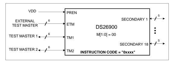
Figure 4-2. Configuration for 1 Master, 20 Secondary Ports
