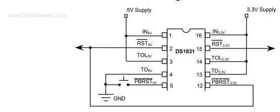
NOTE: The  $\overline{\text{RST}}_{5V}$  output is connected to the IN<sub>3.3V</sub> via a 100 k $\Omega$  resistor in the push-button input and therefore does not require a pull-up resistor (an addition pull up can be used to accelerate responses). If an external pull up is used in this example it must be connected to the 3.3V power supply.
