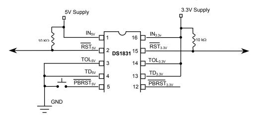
NOTE: If outputs are at different voltages the outputs can not be connected to form a wired AND.
