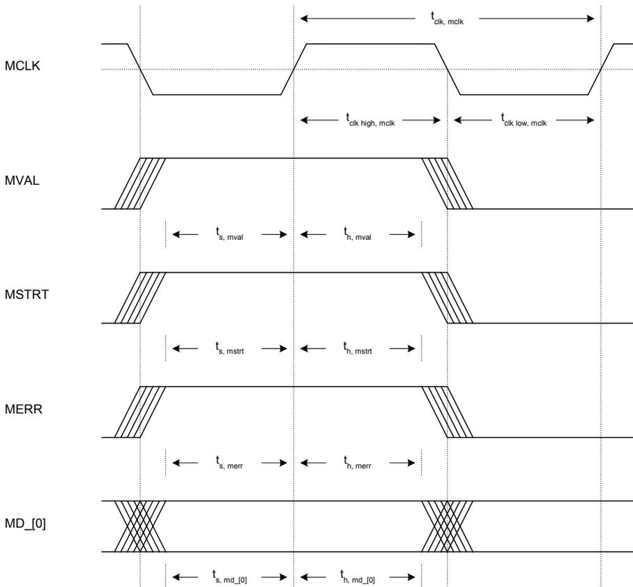
Fig. 4-3: Detailed TS timing (serial mode)
