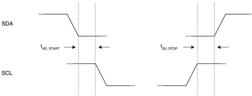
Fig. 4-1: Serial interface start and stop conditions
