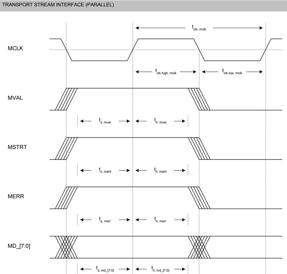
Fig. 4-2: Detailed TS timing (parallel mode)
