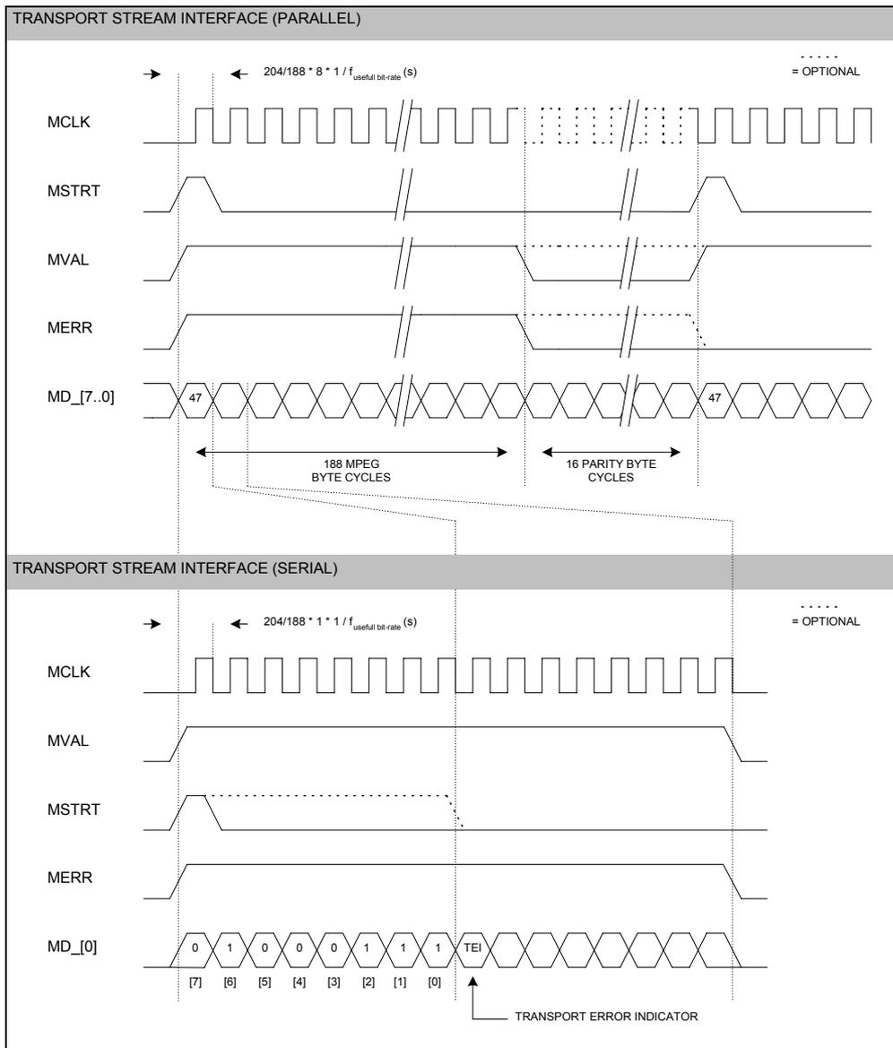
**Fig. 2–8:** Transport Stream interface (with parity bytes)
