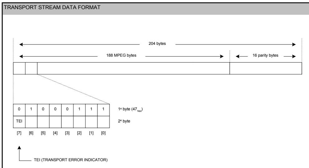
**Fig. 2–6:** Transport Stream data format
