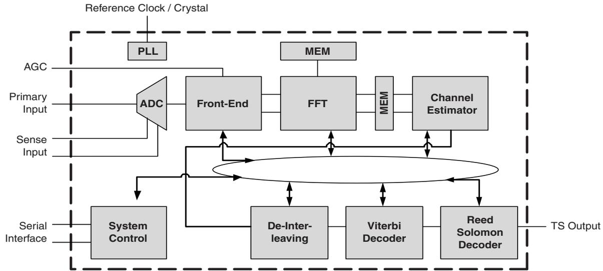
**Fig. 2-1:** Block diagram of the DVB-T demodulator
