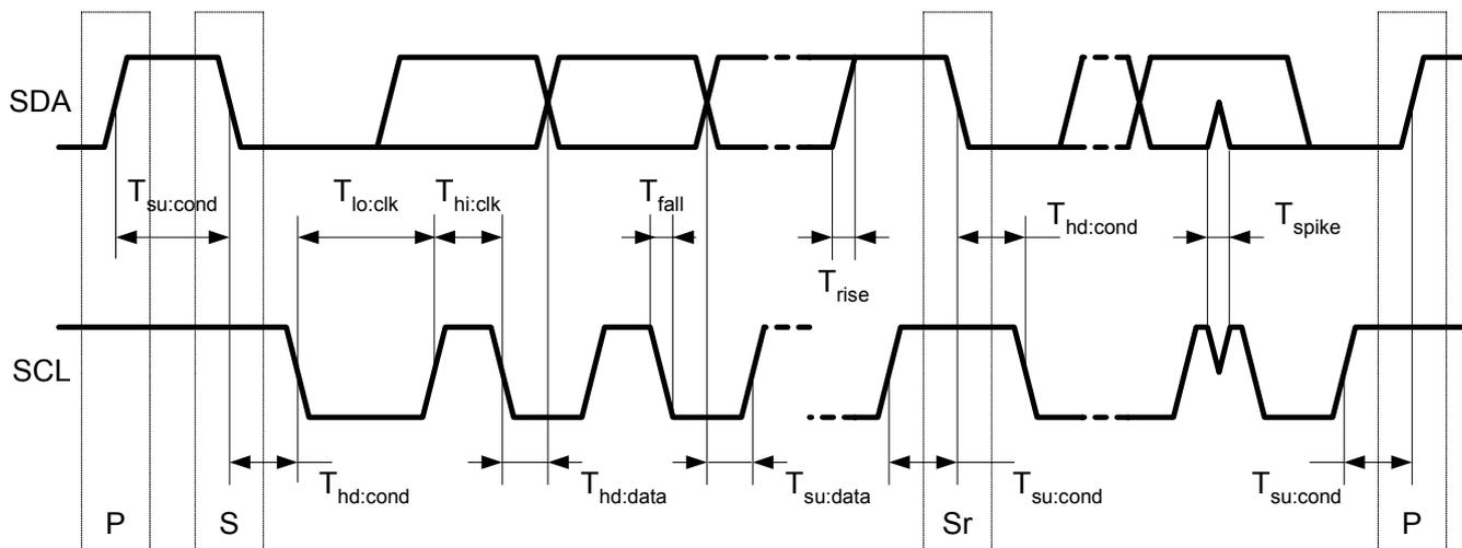
Fig. 3-1: Serial protocol timing diagram P=Stop, S=Start, Sr=Repeated Start.
