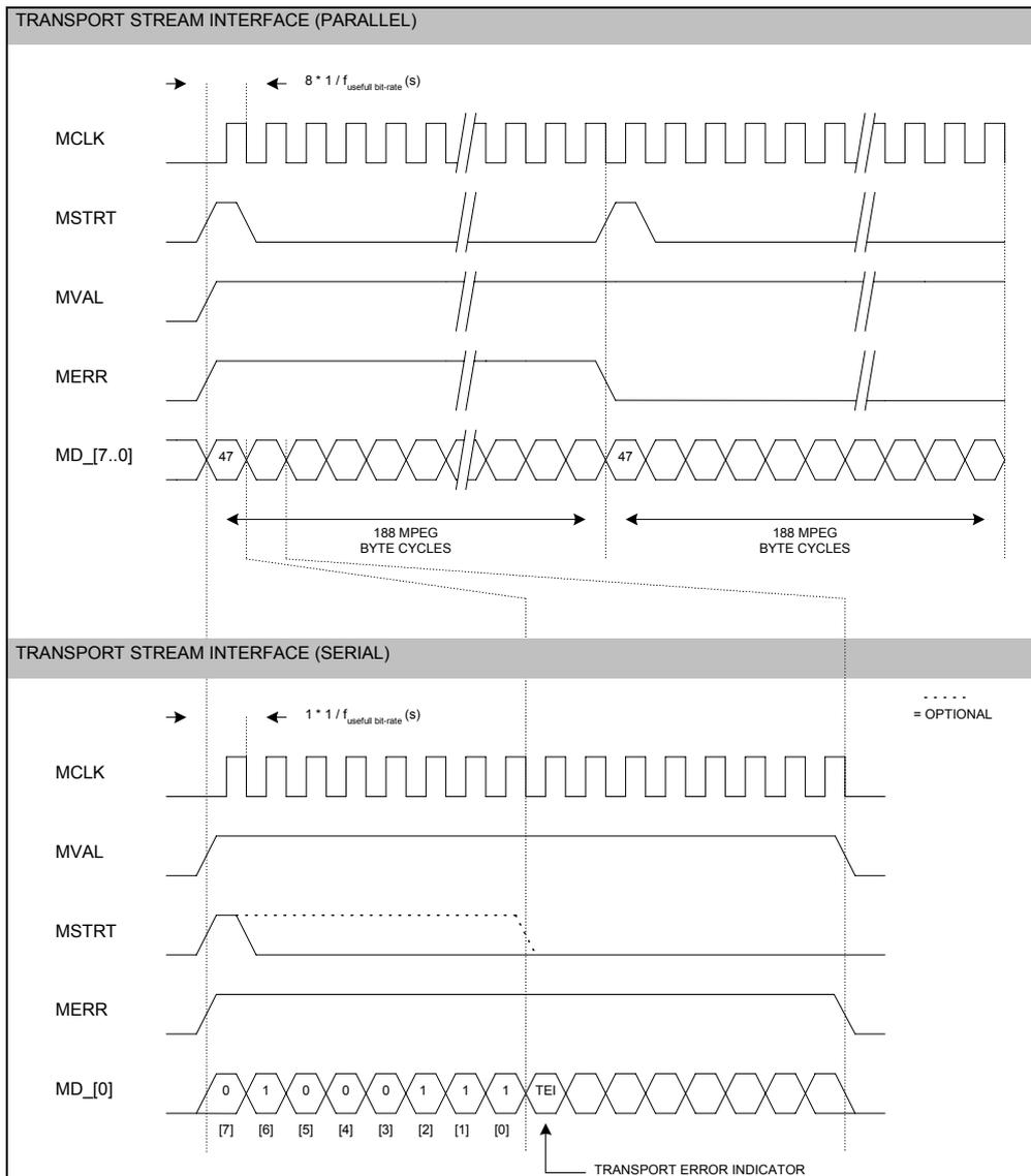
Fig. 2-7: Transport Stream interface (no parity bytes)
