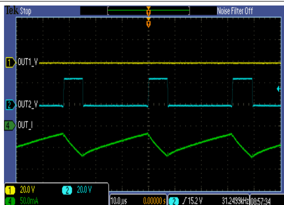
Figure 6. 25% Duty Cycle, Forward Direction
