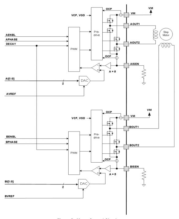
Figure 5. Motor Control Circuitry
