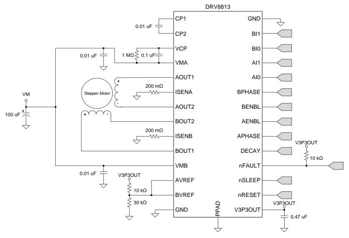
Figure 7. Typical Application Schematic
