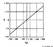
FIGURE 10. Change in Propagation Delay Relative to "True" (Application) Load Minus AC Specified Data Sheet Load
