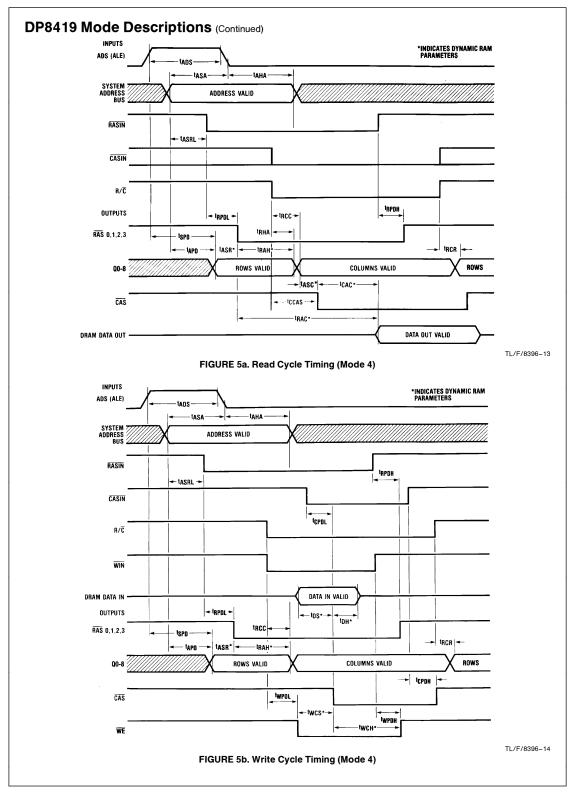
Page or Nibble mode may be performed by toggling  $\overline{CASIN}$  once the initial access has been completed. In the case of page mode the column address must be changed before  $\overline{CASIN}$  goes low to access a new memory location (see *Figure 5c*). Parameter t<sub>CPdif</sub> has been specified in order that users may easily determine minimum  $\overline{CAS}$  pulse widths when  $\overline{CASIN}$  is toggling.
