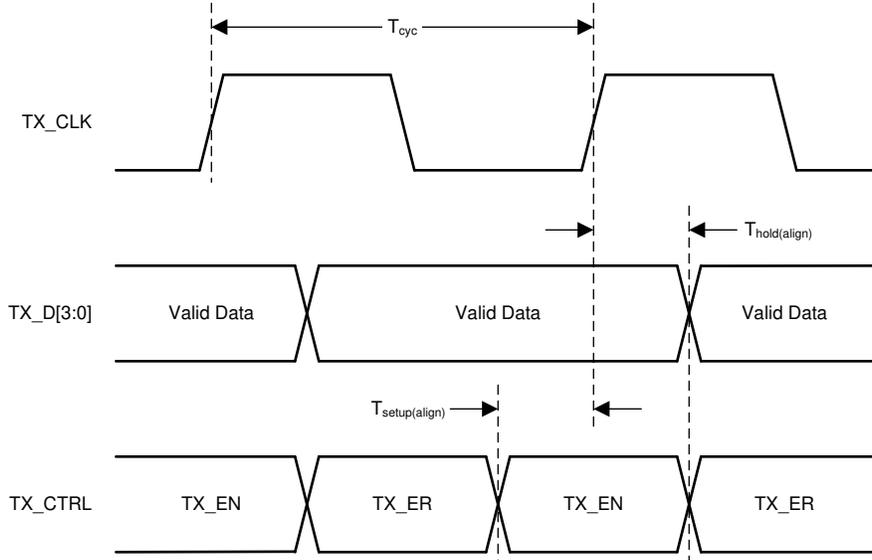
**Figure 6-4. RGMII Transmit Timing (Internal Delay Disabled)**
