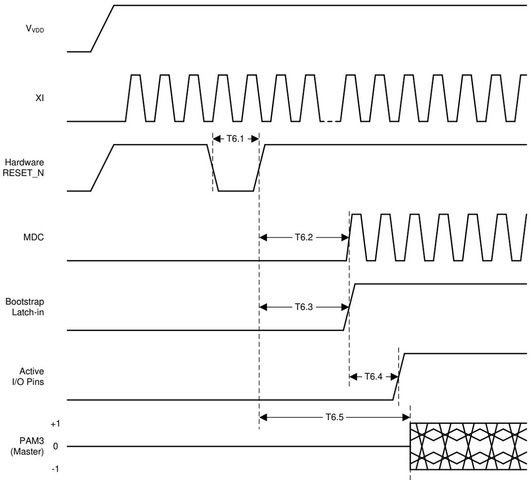
**Figure 6-2. Reset Timing**
