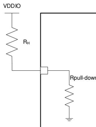
**Figure 7-18. Strap Circuit**
