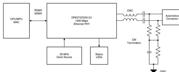
Figure 3-1. Simplified Schematic
