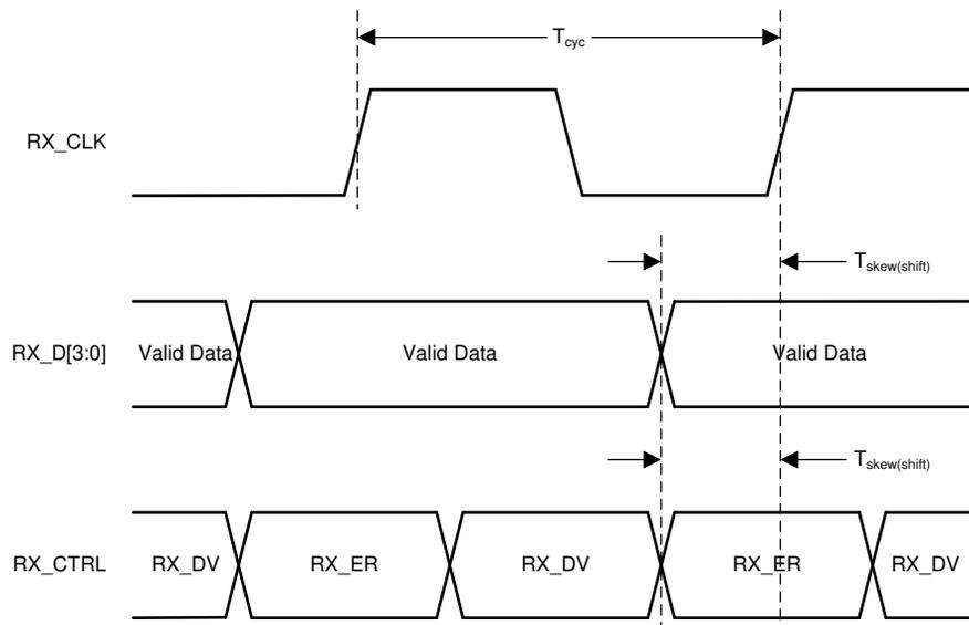
**Figure 6-5. RGMII Receive Timing (Internal Delay Enabled)**
