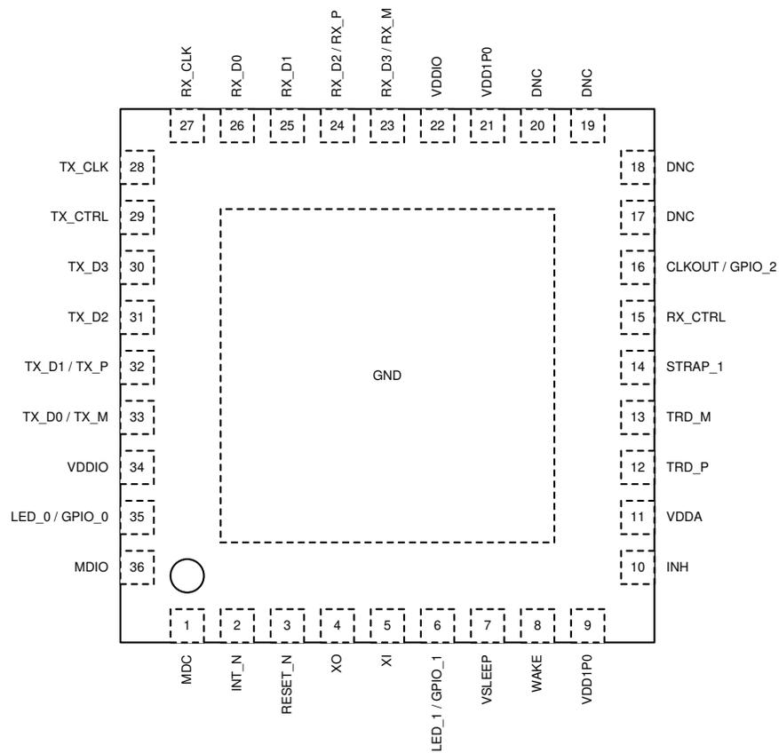
**Figure 5-1. RHA Package 36-Pin VQFN Top View**
