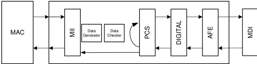
**Figure 7-10. xMII Reverse Loopback With External Data-Gen**
