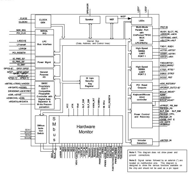
Figure 1 DME1737 Block Diagram
