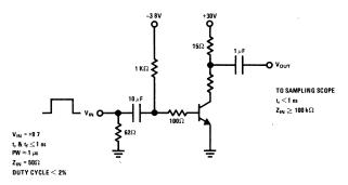
$\text{I}_{\text{C}} \approx 500 \text{ mA}, \, \text{I}_{\text{B1}} \approx 50 \text{ mA}, \, \text{I}_{\text{B2}} \approx -50 \text{ mA}$
