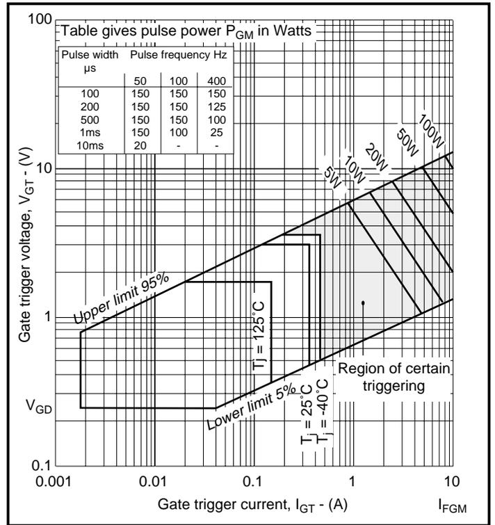
Fig.5 Gate characteristics
