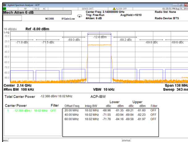
Figure 171. Dual band ACPR Performance in Downlink Band 1 with On-chip PLL
