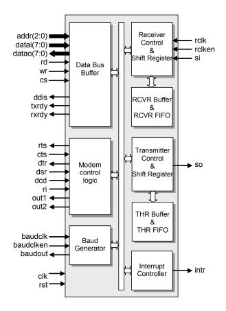
**Baud Generator** - The D16550 contains a programmable 16 bit baud generator that divides clock input by a divisor in the range between 1 and  $(2^{16}-1)$ . The output frequency of the baud generator is 16× the baud rate. The formula for the divisor is:
