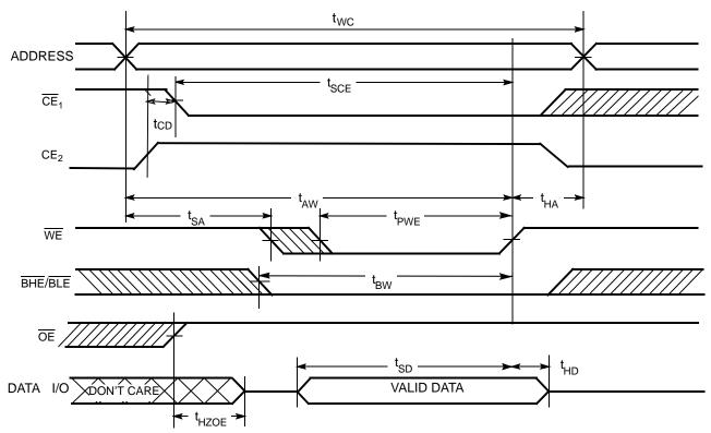
Notes: 20. Data I/O is high-impedance if  $\overline{OE} \ge V_{IH}$ . 21. During the DON'T CARE period in the DATA I/O waveform, the I/Os are in output state and input signals should not be applied.
