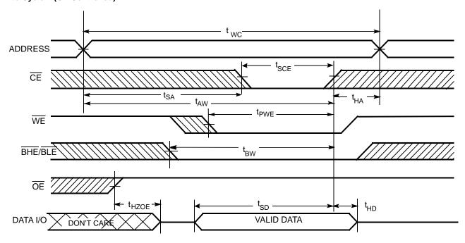
18. Data I/O is high impedance if  $\overline{OE} \ge V_{IH}$ .
