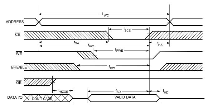
Notes: 17. Data I/O is high impedance if  $\overline{OE} \ge V_{IH}$ . 18. If Chip Enable goes INACTIVE with WE =  $V_{IH}$ , the output remains in a high-impedance state. 19. During the DON'T CARE period in the DATA I/O waveform, the I/Os are in output state and input signals should not be applied.
