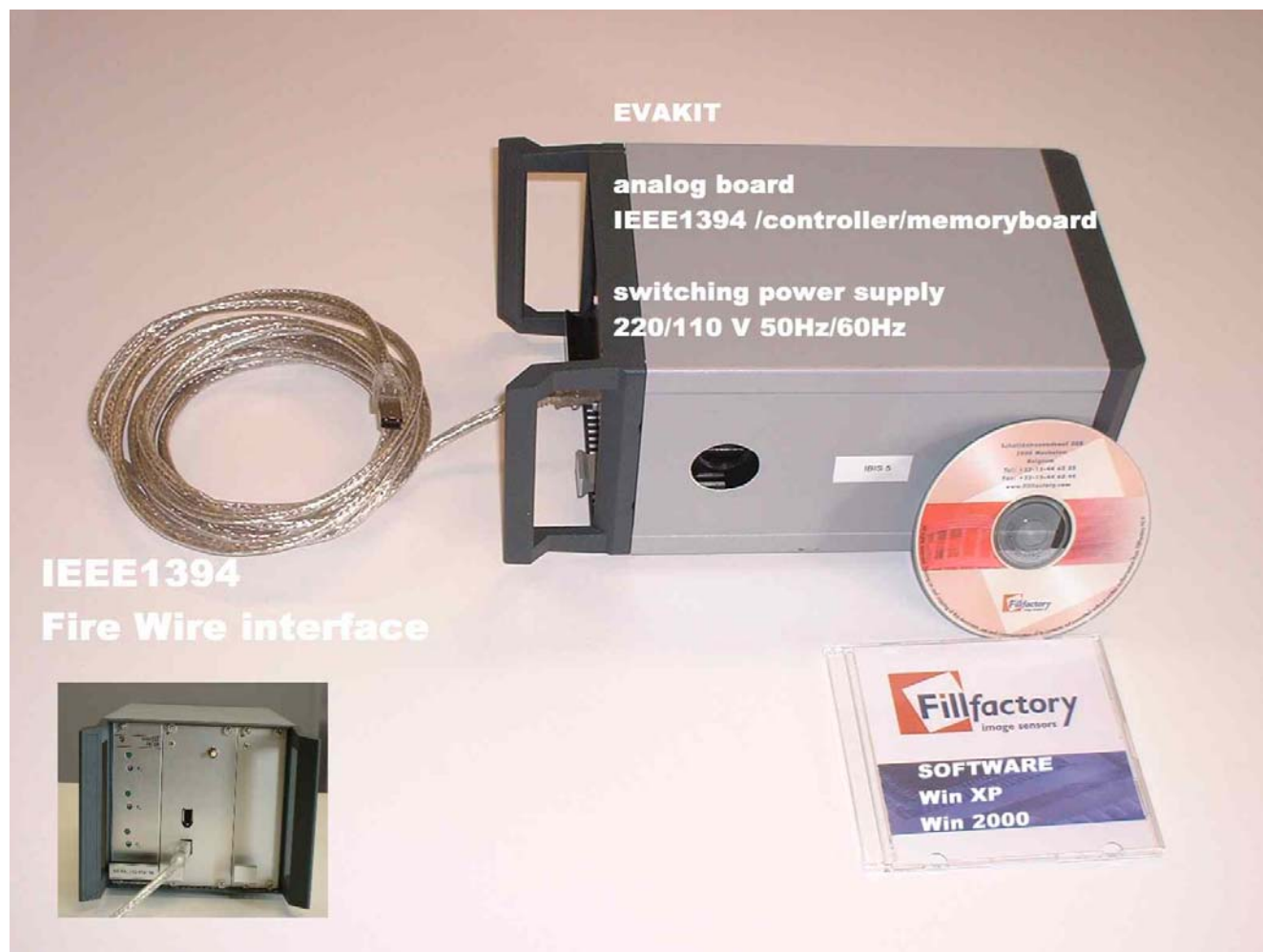
Figure 27. Contents of LUPA 4000 Evaluation Kit
