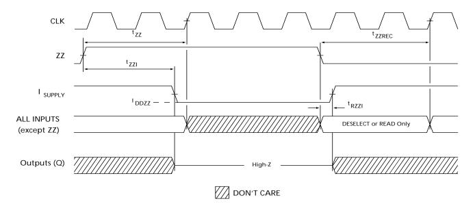
**Notes:**20. Device must be deselected when entering ZZ mode. See Cycle Descriptions table for all possible signal conditions to deselect the device.
