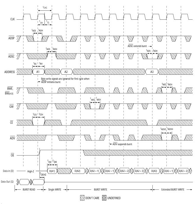
17. Full width write can be initiated by either  $\overline{\text{GW}}$  LOW; or by  $\overline{\text{GW}}$  HIGH,  $\overline{\text{BWE}}$  LOW and  $\overline{\text{BW}}_{[A:D]}$  LOW.
