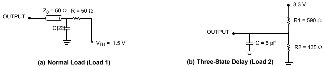
Figure 3. AC Test Loads and Waveforms
