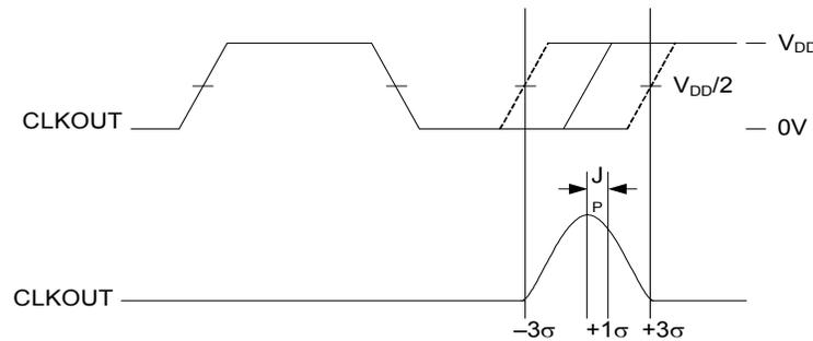
**Figure 6. Cycle to Cycle Jitter**
