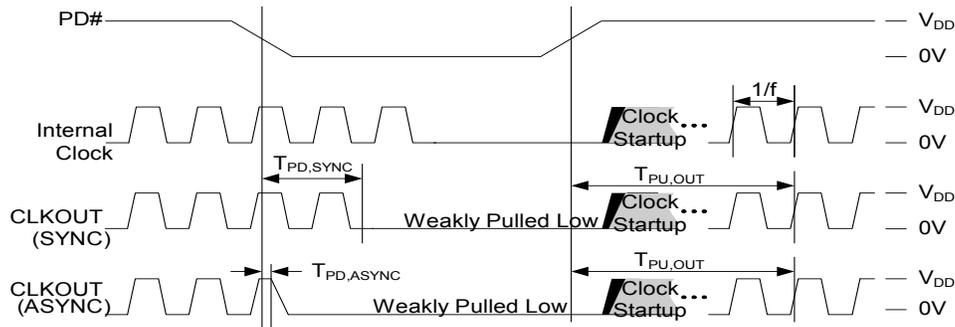
**Figure 9. CLKOUT Enable (Synchronous and Asynchronous Modes) and CLKOUT Disable Timing**
