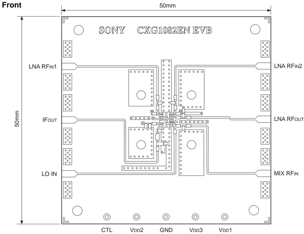
Glass fabric-base 4-layer epoxy board (thickness: 0.2mm × 2)
