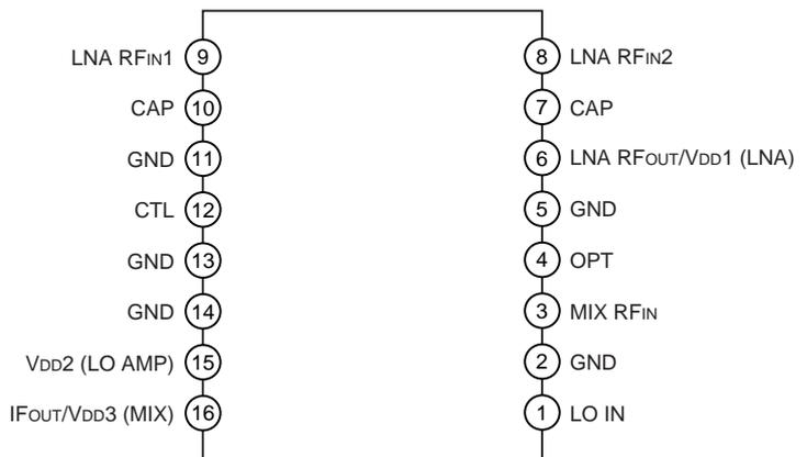
GaAs MMICs are ESD sensitive devices. Special handling precautions are required.
