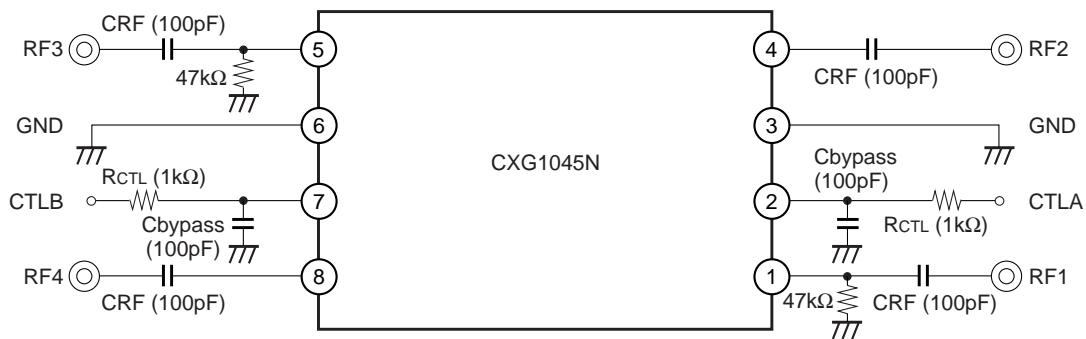
\* Recommended to use DC blocking capacitors (CRF) and bypass capacitors (C bypass).
