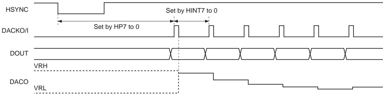
The internally generated digital data DOUT is input to the internal D/A converter, latched by the D/A converter clock input from DACKI, and output from DACO2, 1 and 0 as an analog signal.
