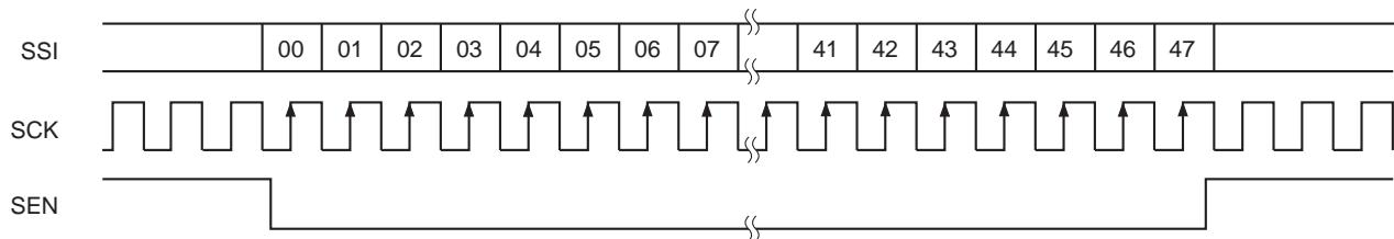
There are two categories of serial interface data: CXD2470R drive control data (hereafter "control data") and electronic shutter data (hereafter "shutter data").
