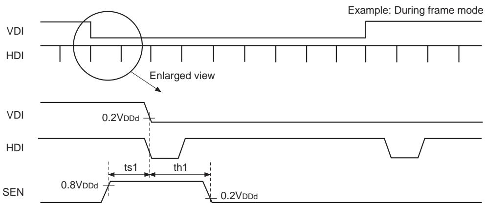
\* Be sure to maintain a constantly high SEN logic level near the falling edge of VDI.
