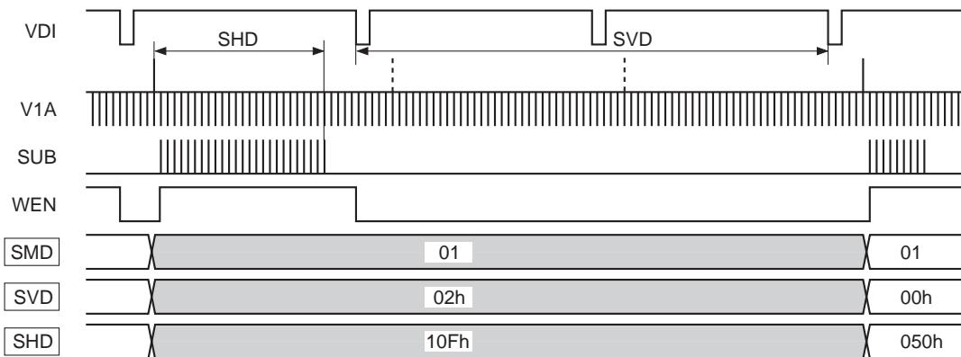
Further, SPL can be used during this mode to specify the SUB output at the desired vertical period during the low-speed shutter period.
