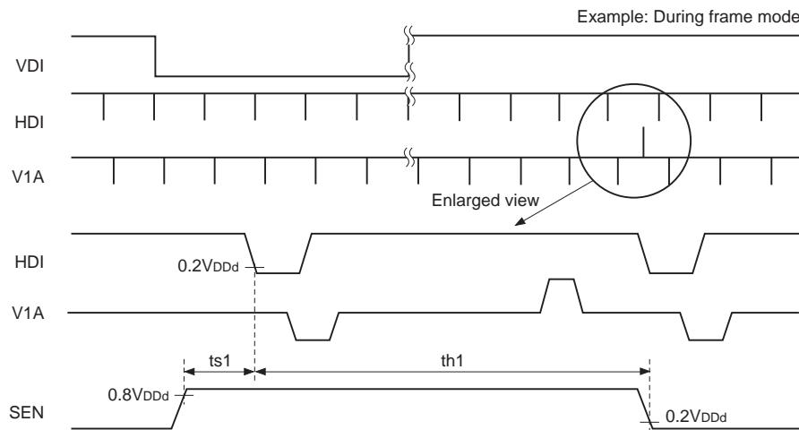
\* Be sure to maintain a constantly high SEN logic level near the falling edge of the HDI in the horizontal period during which V1A/B and V3A/B values take the ternary value and during that horizontal period.
