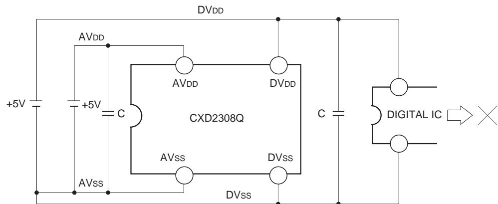
**b. When analog and digital supplies are from common source**
