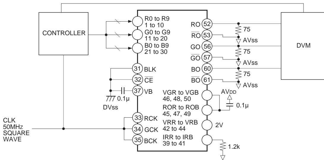
**Propagation Delay Time Measurement Circuit**
