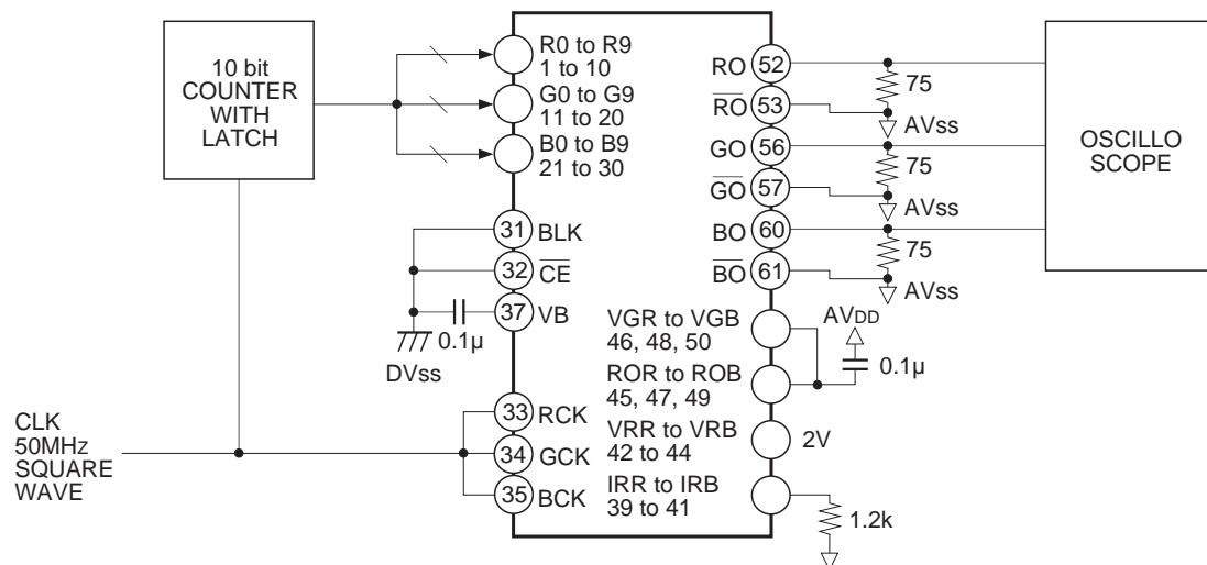
**Setup Time****Hold Time****Glitch Energy****Measurement Circuit**
