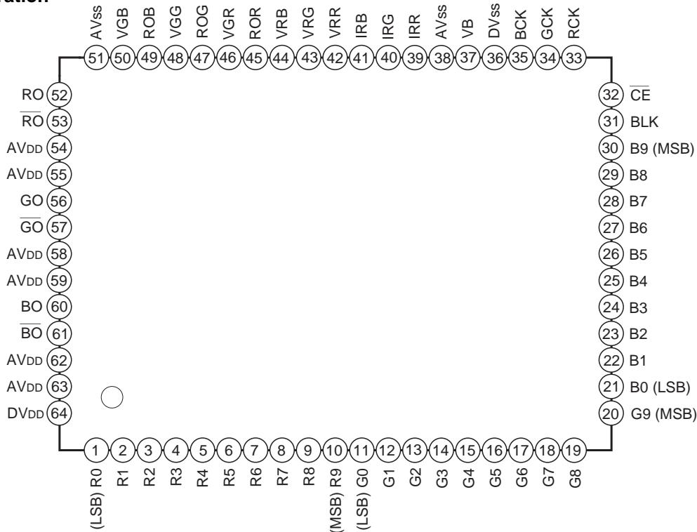
**Pin Description and Equivalent Circuit**
