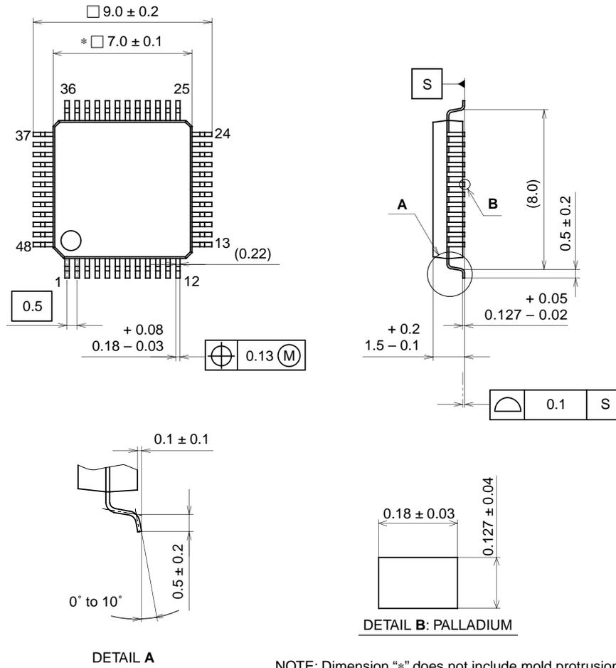
NOTE: Dimension "\*" does not include mold protrusion.
