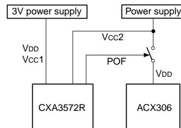
Panel power supply configuration using POF output
