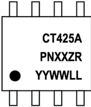
Figure 22: CT425 Device Marking for 8-lead Package
