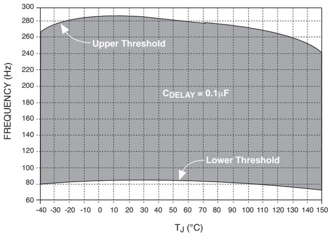
Watchdog Frequency Threshold vs  $C_{DELAY}$
