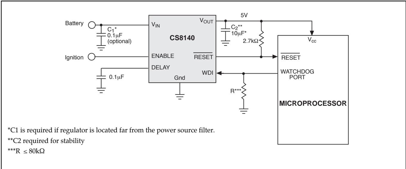
Figure 7. Application Diagram
