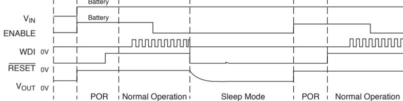
As long as ENABLE is high or ENABLE is low and the Watchdog signal is normal,  $V_{OUT}$  will be at 5V (typ). If ENABLE is low and the Watchdog signal moves outside programmable limits, the output transistor turns off and the IC goes into SLEEP mode. Only the ENABLE circuitry in the IC remains powered up, drawing a quiescent current of  $250\mu\text{A}$ .
