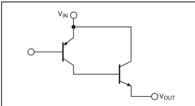
Figure 1: Composite Output Stage of the CS8140/1
