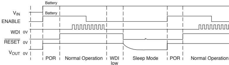
3g: WDI frequency rises above the upper frequency threshold after a normal period of operation; ENABLE = LOW (for the CS8140 only).
