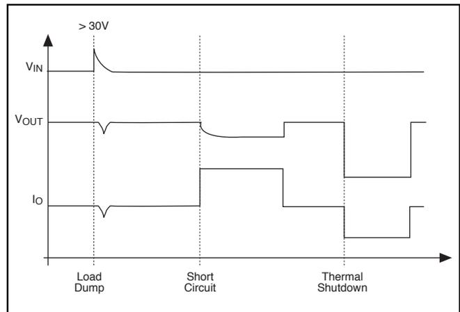
Figure 2: Typical Circuit Waveforms for Output Stage Protection.
