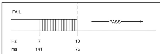
Figure 6: WDI signal for  $C_{\text{Delay}} = 0.82\mu\text{F}$  using CS8141.
