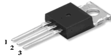
1.Gate 2. Drain 3. Source
