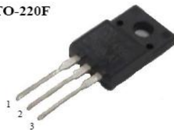
1. Gate 2. Drain 3. Source
