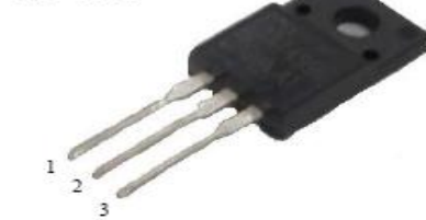
1. Gate 2. Drain 3. Source
