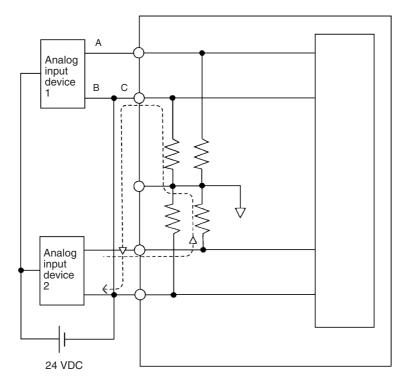
For example, if connected device 2 is outputting 5 V and the same power supply is being used for both devices as shown above, approximately 1/3, or 1.6 V, will be applied to the input for input device 1.
