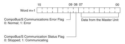
Write the data to be transmitted to the Master Unit in the output word (n+1).
