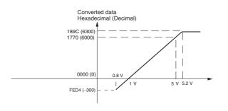
Voltages in the -10 to 10 V range correspond to hexadecimal values F448 to 0BB8 (-3,000 to 3,000). The range of data that can be converted is F31C to 0CE4 hex (-3,300 to 3,300). A negative voltage is expressed as a two's complement.
