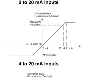
Currents in the 0 to 20 mA range correspond to hexadecimal values 0000 to 1770 (0 to 6,000). The range of data that can be converted is FED4 to 189C hex (-300 to 6,300). A negative current is expressed as a two's complement.
