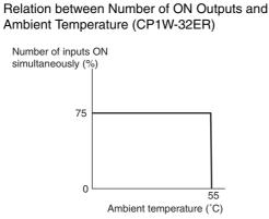
According to the ambient temperature, there are restrictions on power supply voltage and output load current for the CPU Units connected with the Expansion I/O Units (CP1W-8ER/16ER/20EDR1/ 32ER/40EDR). Use the PLC in the range of the power supply voltage and output load current as show below.
