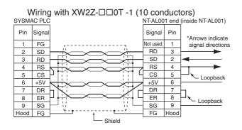
**Note** The hood (FG) is internally connected to the ground terminal (GR) on the CPU Unit. Therefore, FG is grounded by grounding the ground terminal (GR) on the power supply terminal block.
