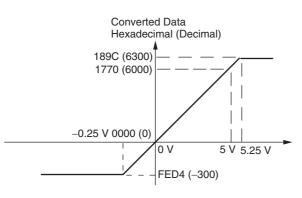
Voltages in the 0 to 5 V range correspond to hexadecimal values 0000 to 1770 (0 to 6,000). The range of data that can be converted is FED4 to 189C hex (-300 to 6,300). A negative voltage is expressed as a two's complement.
