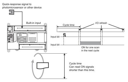
**Note** The user setting in the PLC Setup determines if each input is a quick-response input, normal input, interrupt input, or high-speed counter input.
