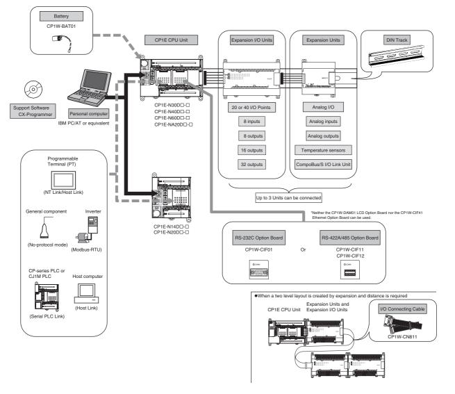
The system configuration when using a CP1E N/NA-type CPU Unit is shown below.
