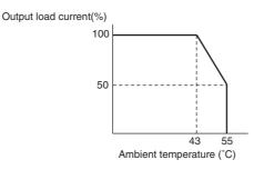
• CP1W-32ER's maximum number of simultaneously ON output points is 24 (75%).
