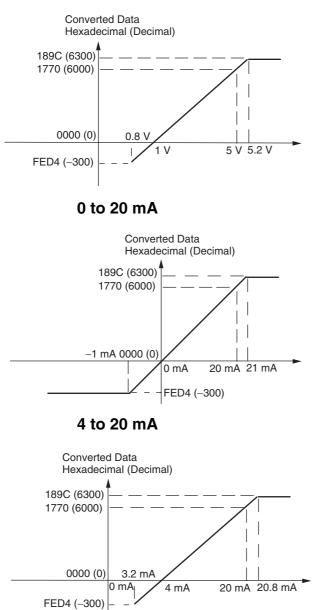
Voltages in the 1 to 5 V range correspond to hexadecimal values 0000 to 1770 (0 to 6,000). The range of data that can be converted is FED4 to 189C hex (-300 to 6,300).
