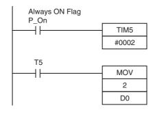
TIM 5 will start as soon as power turns ON. After 0.1 to 0.2 s (100 to 200 ms), the input for TIM 5 will turn ON, and the converted data from analog input 0 that is stored in CIO 2 will be transferred to D0.
