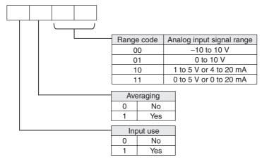
• The Analog Input Unit will not start converting analog I/O values until the range code has been written.
