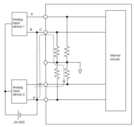
Example: If connected device 2 is outputting 5 V and the same power supply is being used for both devices as shown above, approximately 1/3, or 1.6 V, will be applied to the input for input device 1.
