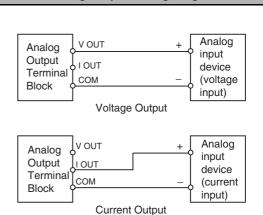
**Analog Output Wiring Diagram**
