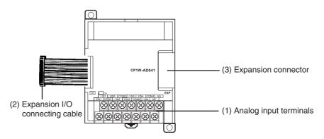
(1)Analog Input Terminals Connected to analog output devices.
