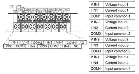
Note When using current inputs, voltage input terminals must be short-circuited with current input terminals.
