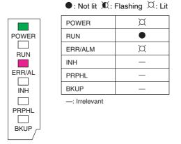
There may be a CPU error or a fatal error if operation stops (i.e., the RUN indicator turns OFF) and the ERR/ALM indicator lights.
