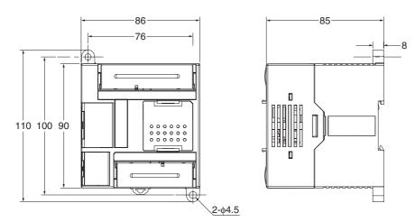
CPU Units with 30 I/O Points (CP1E-□30D□-□) CPU Units with Built-in Analog and 20 I/O Points (CP1E-NA20D□-□)
