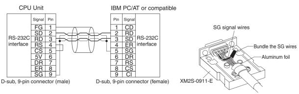
Note The hood (FG) is internally connected to the ground terminal (GR) on the CPU Unit.
