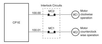
A circuit like the one shown in the diagram on the left is required to prevent outputs MC1 and MC2 from both being ON at the same time even if both PLC outputs CIO 100.00 and CIO 100.01 are both ON.
