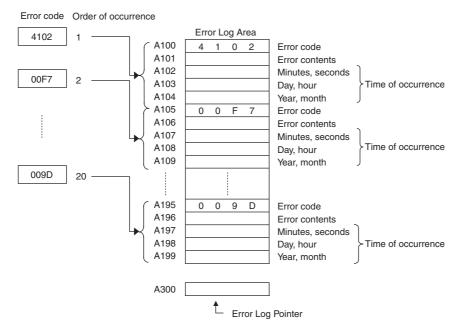
**Note** CP1E E-type CPU Units do not support the clock function, so the time of occurrence cannot be confirmed. The display is always 01-01-01 01:01:01 Sunday.
