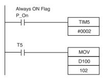
TIM 005 will start as soon as power turns ON. After 0.1 to 0.2 s (100 to 200 ms), the Completion Flag for TIM 005 will turn ON, and the data stored in D100 will be moved to CIO 102 as the conversion data for analog output 1.
