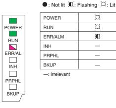
Information on the non-fatal errors can be obtained from the Errors Tab Page of the CX-Programmer's PLC Errors Window.
