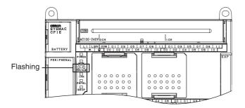
When the ERR/ALM indicator flashes, connect the CX-Programmer to the peripheral USB port and read the error messages.
