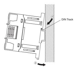
**3** Press in all of the DIN Track mounting pins to securely lock the Units in place.
