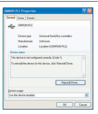
2 Click the **Reinstall Driver** Button. The Hardware Update Wizard Dialog Box will be displayed. Install the driver software using the procedure described in *4-2-2 Installing the USB Driver*
