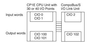
The input word (m+1) contains the data from the Master Unit and the CompoBus/S communications status.
