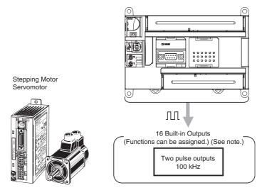
Note The instruction used to control each output determines whether it is used as a normal output, pulse output, or PWM output.
