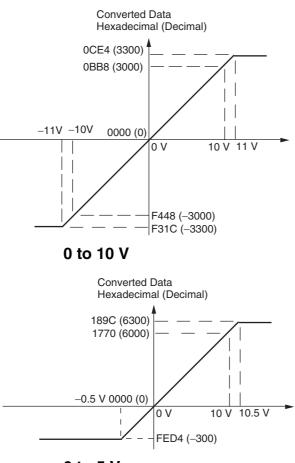
Voltages in the -10 to 10 V range correspond to hexadecimal values F448 to 0BB8 (-3,000 to 3,000). The range of data that can be converted is F31C to 0CE4 hex (-3,300 to 3,300). A negative voltage is expressed as a two's complement.
