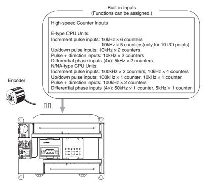
**Note** The user setting in the PLC Setup determines if each input is a quick-response input, normal input, interrupt input, or high-speed counter input.
