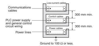
• If the I/O wiring and power cables must be placed in the same duct, they must be shielded from each other using grounded steel sheet metal.
