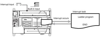
**Note** The user setting in the PLC Setup determines if each input is a quick-response input, normal input, interrupt input, or high-speed counter input.
