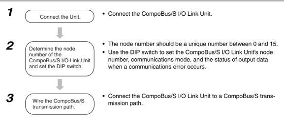
1 Connect the CompoBus/S I/O Link Unit to the CPU Unit.
