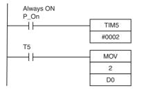
TIM5 is started when the power is turned ON. After 0.1 to 0.2 s (100 to 200 ms) elapses, the TIM5 contact turns ON and the analog input 1 conversion data stored in CIO 2 is transferred to D0.
