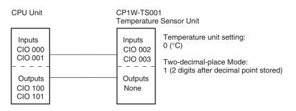
In this example, 100 times the temperature data for temperature input 0 (input to CIO 002) is stored in binary form in D100 to D102.
