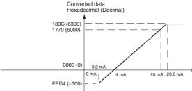
Currents in the 4 to 20 mA range correspond to hexadecimal values 0000 to 1770 (0 to 6,000). The range of data that can be converted is FED4 to 189C hex (-300 to 6,300). Current in the range of 3.2 to 4 mA is expressed as a two's complement.
