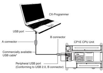
\* Commercially available USB cable: 5 m max., for USB 2.0.
