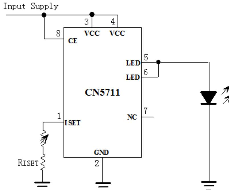
Figure 5 A Potentiometer to Dim the LED
