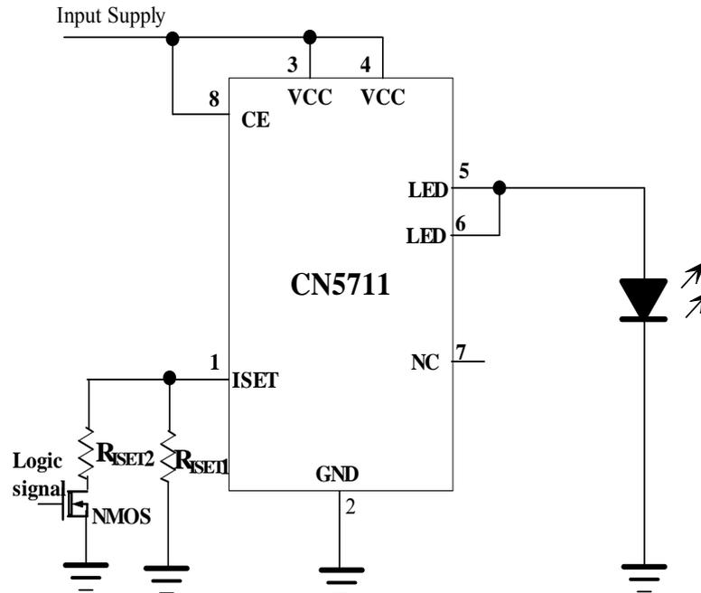
Figure 4 A logic signal to Dim LED
