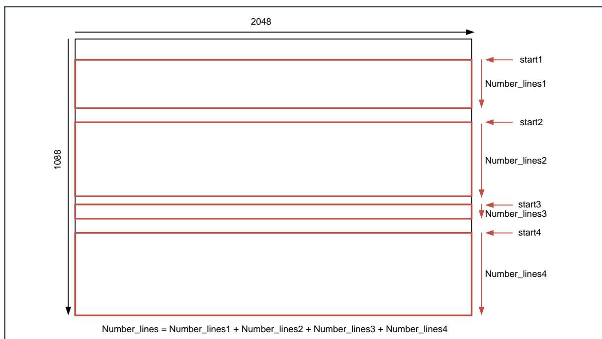
Figure 67: Example of 4 Multiple Frames Read-Out
