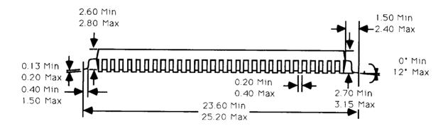
NOTE: Dimensions for the QFP package are in millimeters.
