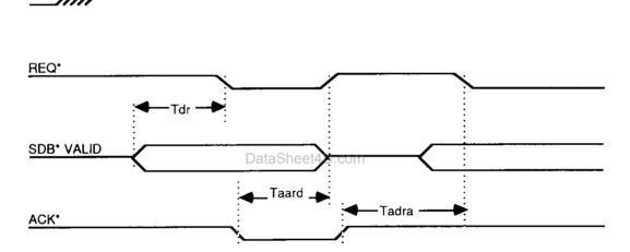
NOTE: The MOE\* signal (Pin 15) will be continuously asserted low every unused BUFCLK\* cycle while waiting for the falling (leading) edge of the SCSI ACKNOWLEDGE signal (ACK\* — Pin 70).
