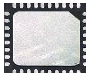
36 lead 6x5 mm QFN package
