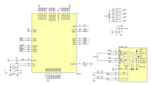
Note: Due to space limitations, the circuit of the power supply and decoupling capacitors near the 3.3V and 1.8V pins is omitted in the figure, which must be added when designing the circuit. The detailed circuit reference file: CH9121PCB (please download in our official website).
