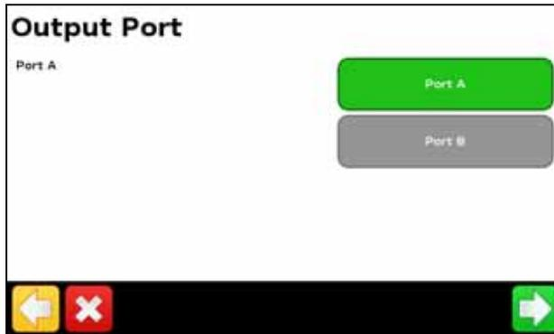
**Note** – Do not configure the display to output NMEA messages on the same port that your controller is connected to.
