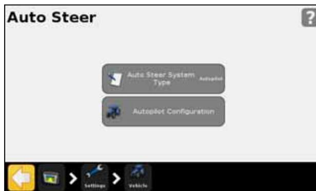
*Note* – If the Autopilot Configuration button does not appear, tap Auto Steer System Type and then select Autopilot for your controller.
