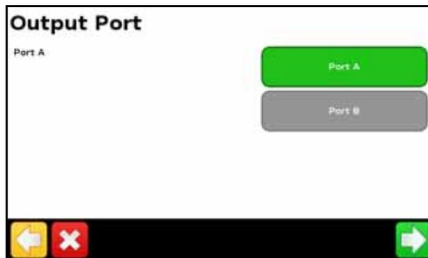
2. On the CFX-750 display, make sure that Output Port matches the port on the display that the controller is connected to (COM or AUX).
