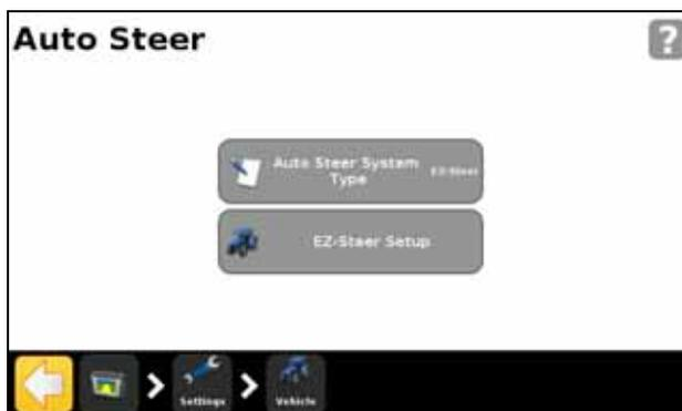
**Note** – If the *EZ-Steer Setup* button does not appear, tap *Auto Steer System Type* and then select *EZ-Steer* for your controller.
