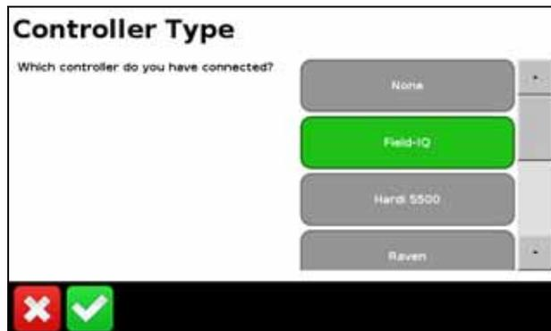
**Note** – To access all of the available *Controller Type* options (apart from *None* and *Field-IQ*) you must have a VRA unlock code. To obtain a VRA unlock code, contact your Trimble reseller.
