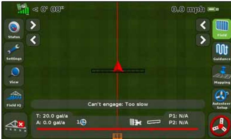
The guidance screen displays a mix of text and icons that provide operating information and access to various system functions. The availability of the text and icons depends on the set up of your system. For example, some icons are not available while you are using an auto steer system.
