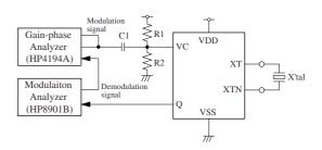
C1 = 20µF, R1 = R2 = 100M $\Omega$ , V<sub>DD</sub> = 3.3V VC modulation signal: 100Hz to 100kHz, 3.3Vp-p
