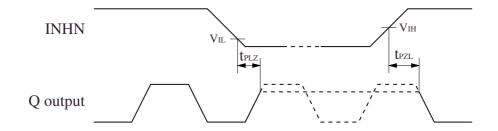
INHN input waveform  $tr = tf \le 10ns$
