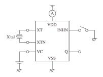
$V_C = 0.5V_{DD}$ , INHN = open, crystal oscillation
