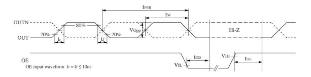
$\begin{array}{l} DUTY1=100t_W\!/t_{PER}~(\%) @\ crossing \ point\\ DUTY2=100t_W\!/t_{PER}~(\%) @\ 50\% \ waveform \end{array}$
