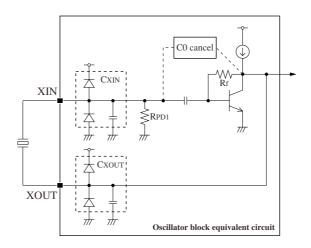
The CF5036 series oscillator circuit has a C0 cancel circuit built-in to improve the oscillator margin. If power is applied when there is an open circuit between XIN and XOUT, self oscillation may occur, which is not abnormal. Users should confirm that the oscillator operates normally when a crystal unit is connected.
