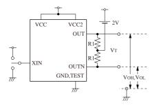
$\begin{array}{l} \text{R1: 49.9} \Omega \\ \text{XIN} = \text{HIGH: OUT} = \text{HIGH} \\ \text{XIN} = \text{LOW} : \text{OUT} = \text{LOW} \\ \end{array}$
