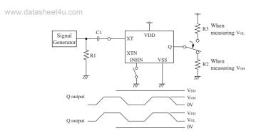
1Vp-p, 10MHz sine wave input signal
