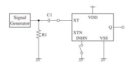
1Vp-p, 10MHz sine wave input signal
