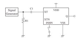
2Vp-p, 10MHz sine wave input signal
