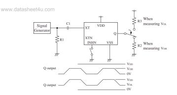
2Vp-p, 10MHz sine wave input signal
