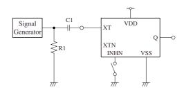
2Vp-p, 10MHz sine wave input signal
