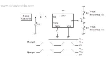
2Vp-p, 10MHz sine wave input signal
