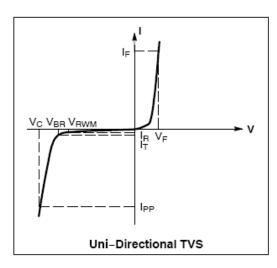
ELECTRICAL CHARACTERISTICS (Ta = 25°C unless otherwise noted, V<sub>F</sub> = 0.9 V Max. @ I<sub>F</sub> = 10mA for all types)
