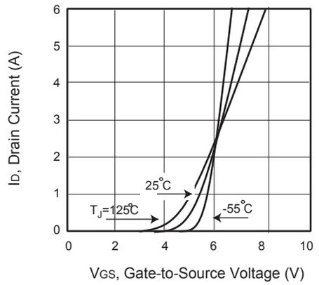
**Figure 2. Transfer Characteristics**
