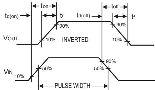
**Figure 10. Switching Waveforms**
