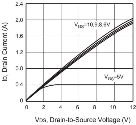
**Figure 1. Output Characteristics**
