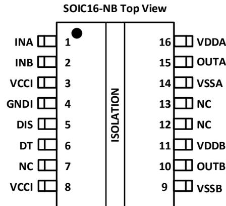
Figure 6-1. The CA-IS3221-Q1 Pin Configuration (SOIC16 Narrow Package)
