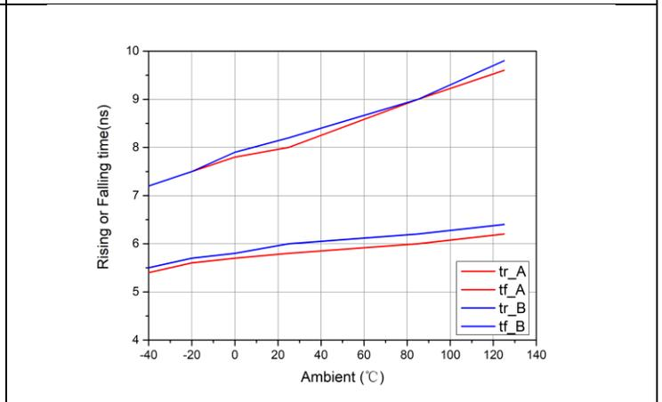
Figure 7-6 Rise time & Fall time VS. Temperature (C<sub>load</sub>=1.8nF)
