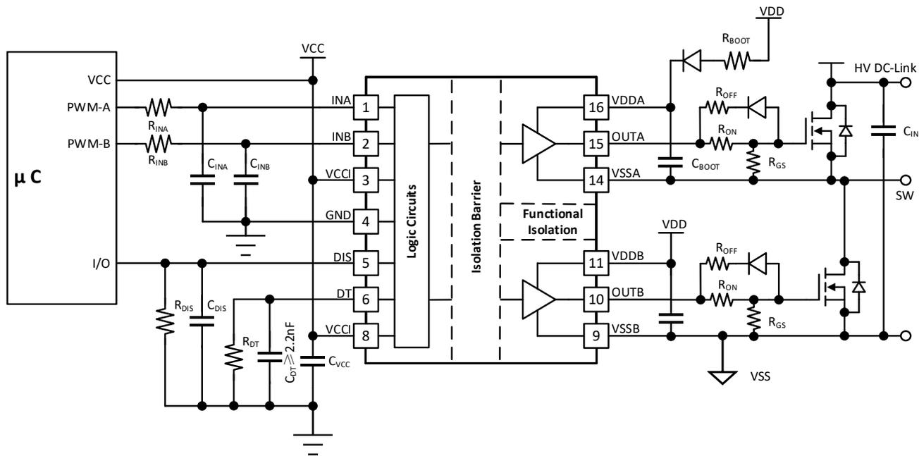
Figure 10-1. Typical application circuit for CA-IS3221-Q1
