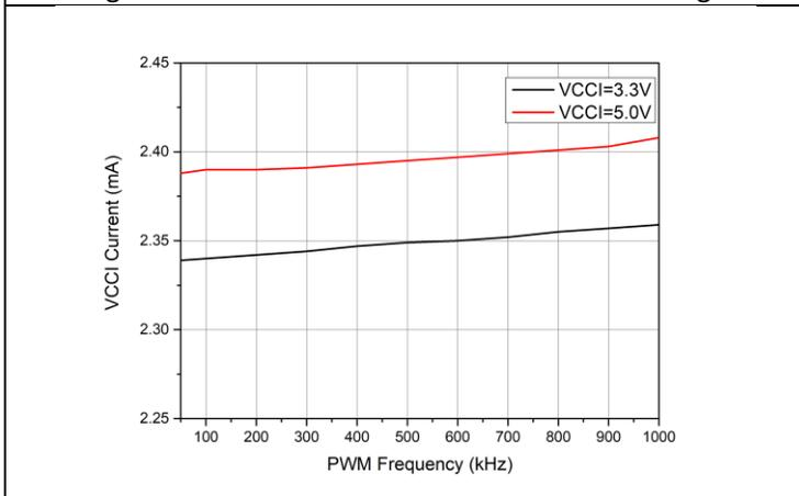
Figure 7-3 VCCI operating current VS. PWM frequency
