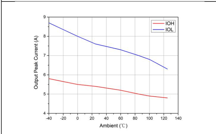
Figure 7-5 Output peak current VS. Temperature (C<sub>load</sub>=180nF)
