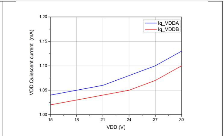
Figure 7-2 VDD Quiescent current VS. VDD voltage
