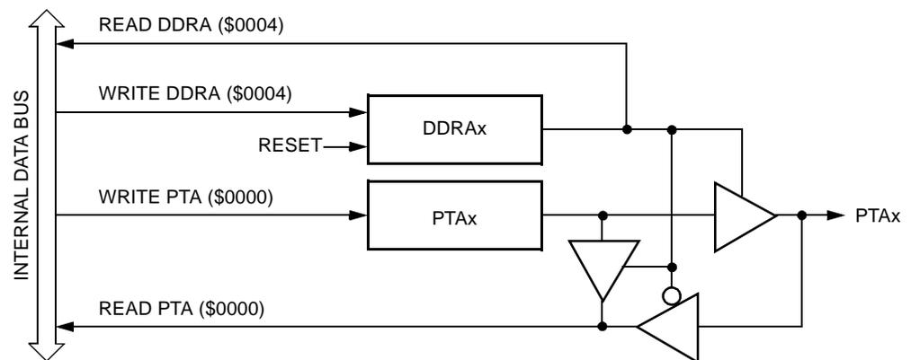
Figure 19-3. Port A I/O Circuit
