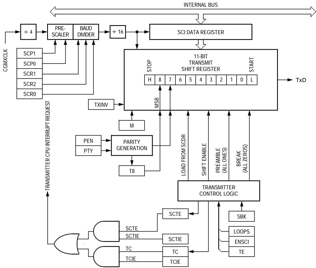
Figure 15-4. SCI Transmitter
