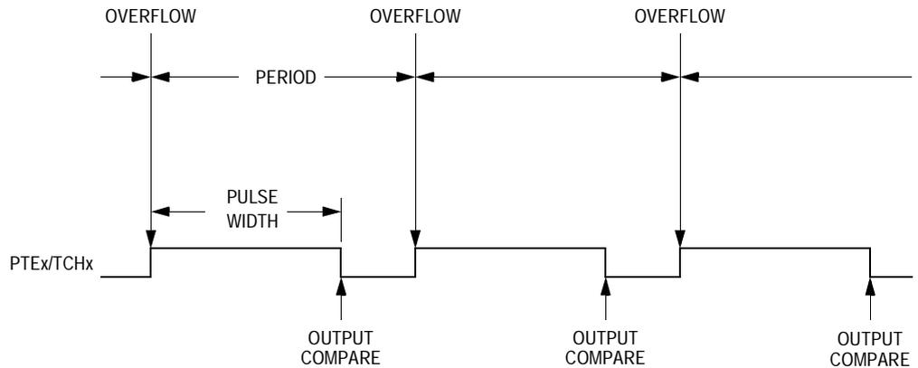
Figure 22-3. PWM Period and Pulse Width
