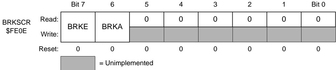
Figure 10-2. Break Status and Control Register (BRKSCR)
