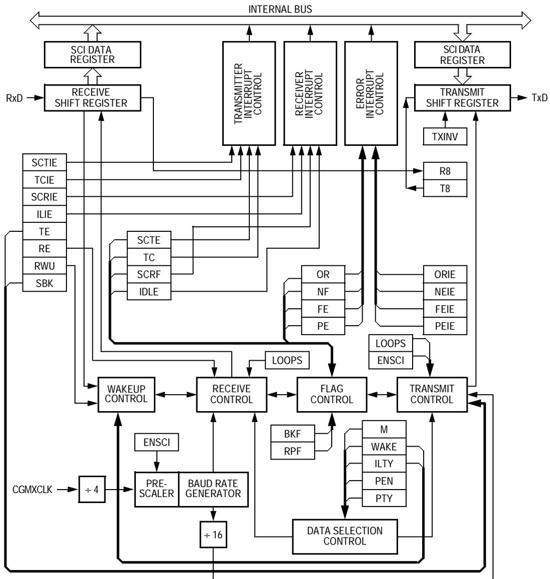
Figure 15-1. SCI Module Block Diagram
