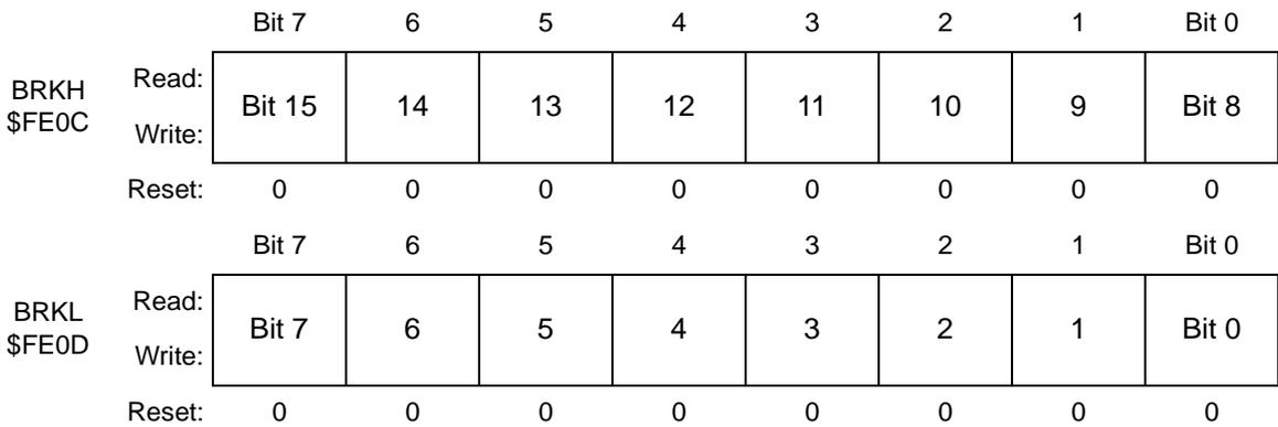
**Figure 10-3. Break Address Registers (BRKH and BRKL)**
