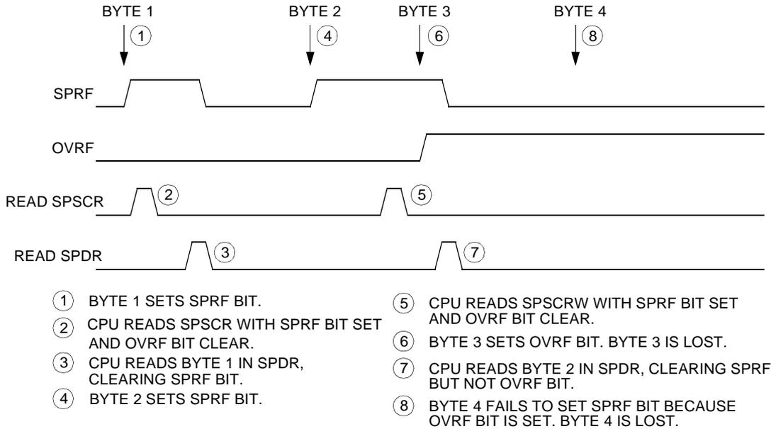
**Figure 16-7. Missed Read of Overflow Condition**
