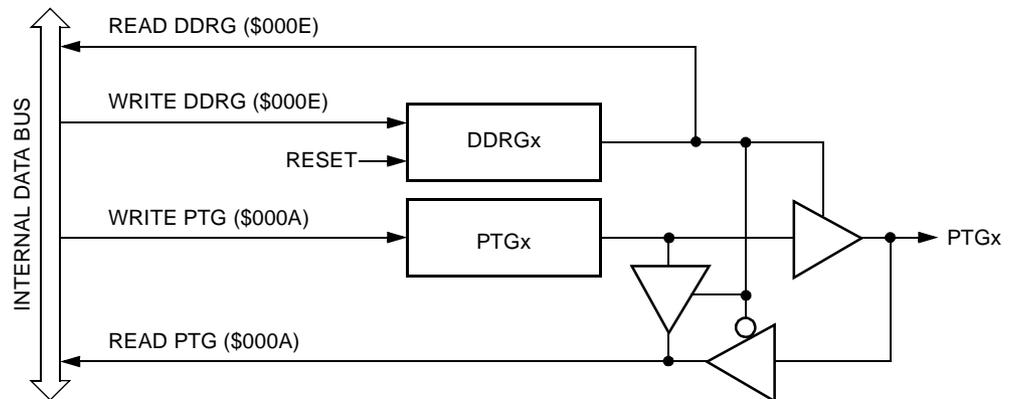
Figure 19-21. Port G I/O Circuit
