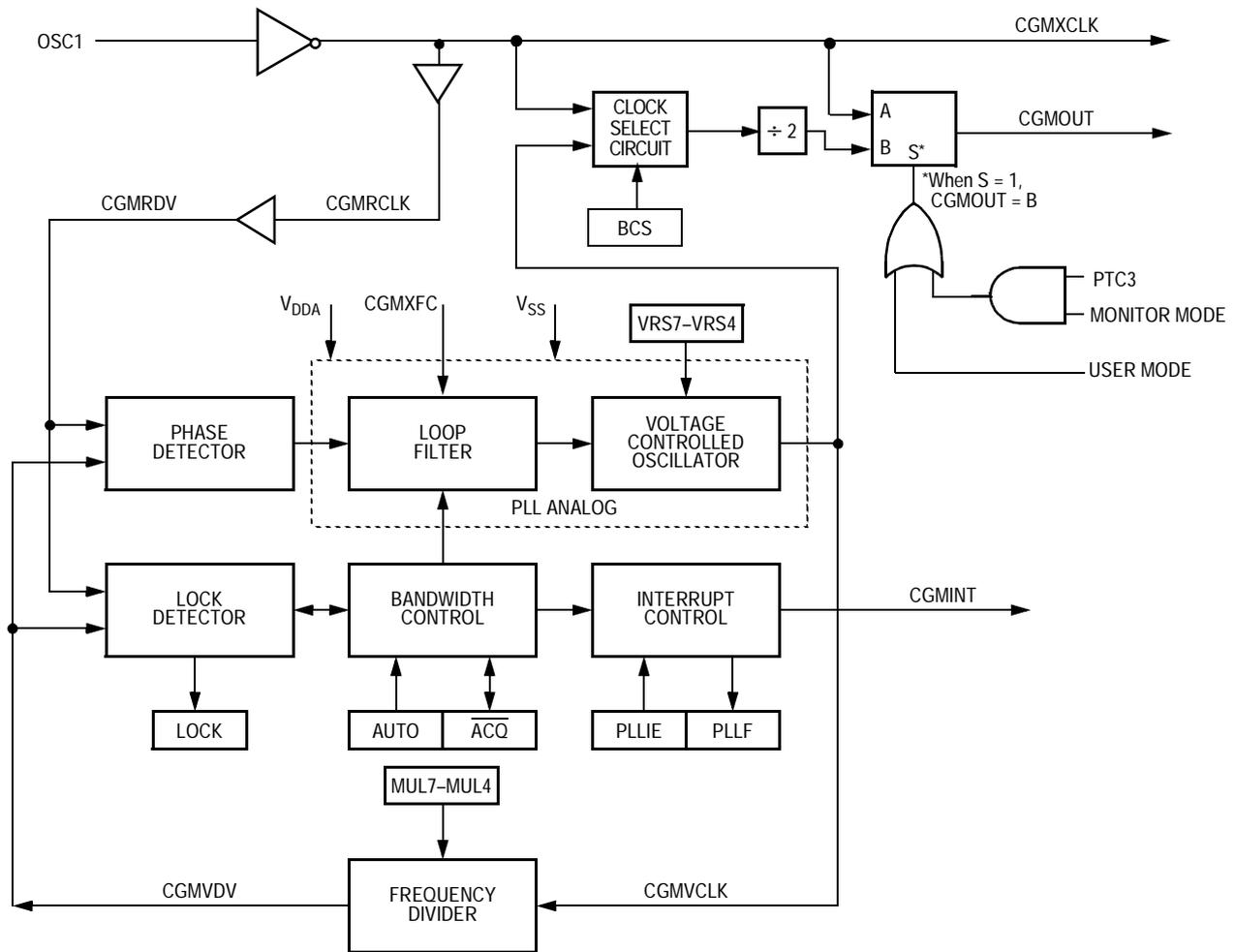
**Figure 8-1. CGM Block Diagram**
