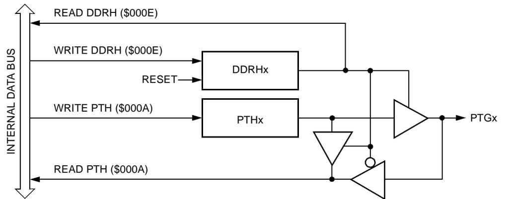
Figure 19-24. Port H I/O Circuit
