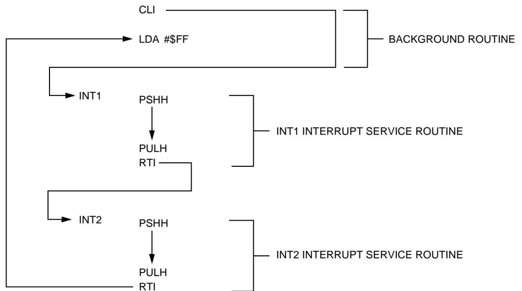
Figure 7-9. Interrupt Recognition Example
