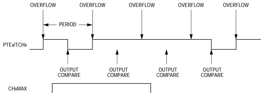
**Figure 17-8. CHxMAX Latency****17.9.5 TIMB Channel Registers**
