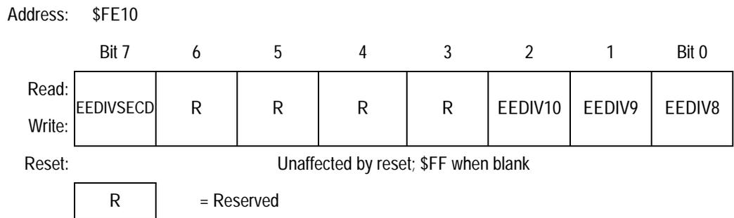
**Figure 5-7. EEPROM Divider Non-Volatile Register High (EEDIVHNVR)**
