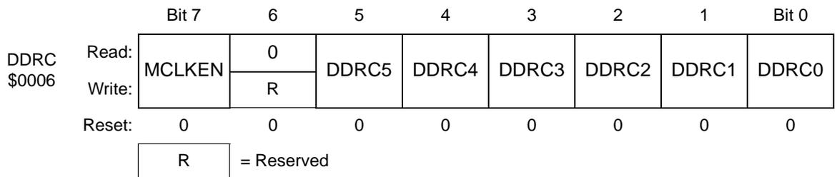
Figure 19-8. Data Direction Register C (DDRC)
