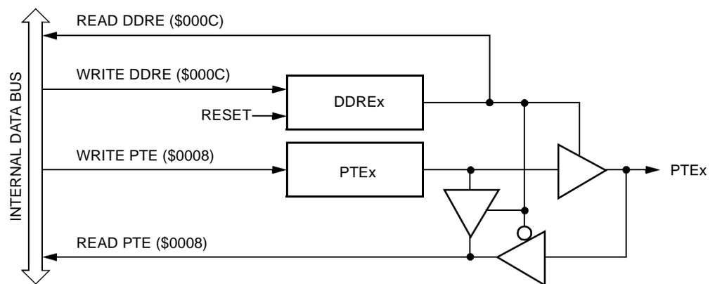
Figure 19-15. Port E I/O Circuit
