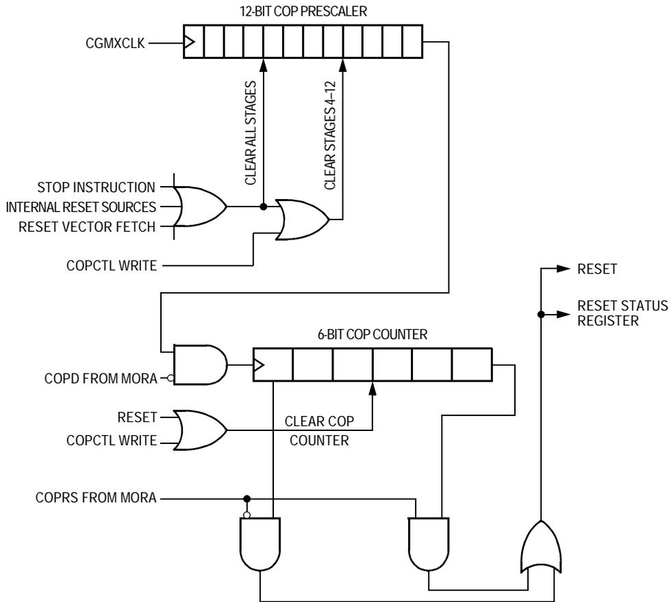
Figure 12-1. COP Block Diagram
