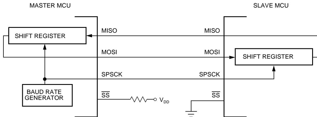
Figure 16-3. Full-duplex Master-Slave Connections
