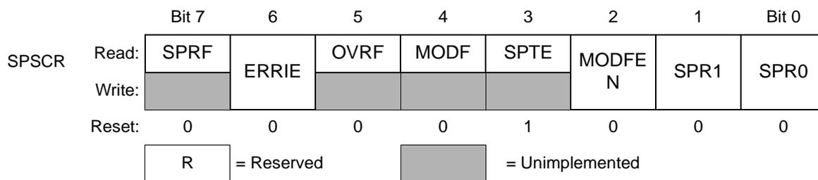
**Figure 16-13. SPI Status and Control Register (SPSCR)**
