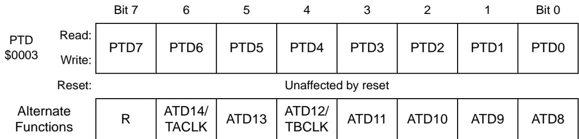
Figure 19-10. Port D Data Register (PTD)
