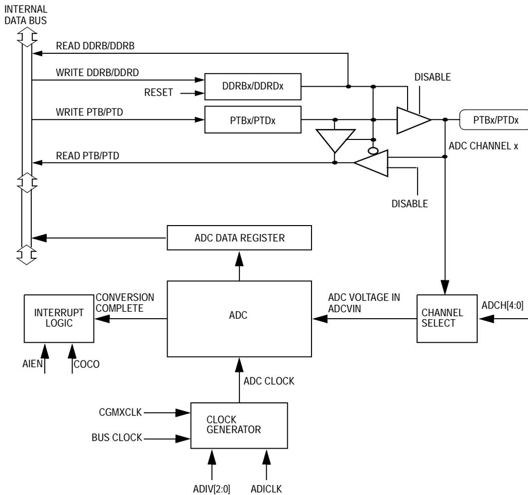
**Figure 23-1. ADC Block Diagram**
