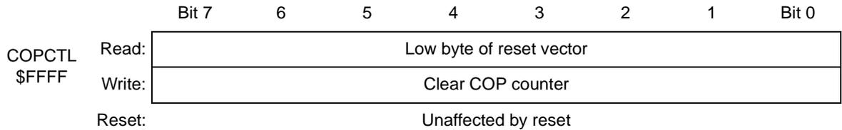
**Figure 12-2. COP Control Register (COPCTL)**
