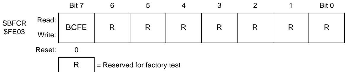
**Figure 7-17. SIM Break Flag Control Register (SBFCR)**
